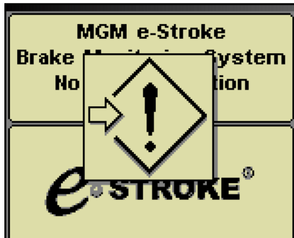
Figure 4: Display Communication Failure Screen
